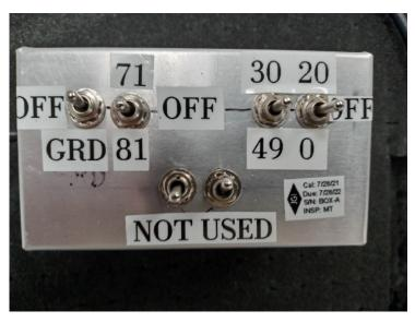
Fig. 5 Fuel Indicator Test Box
