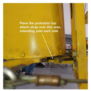
Once attached to the lower rudder hinge bracket as described above, hand tighten the screws to clamp to the hinge bracket. Ensure that the strap forward edge is against the hinge bracket as shown in Fig.3 below.
